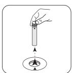
Remove vial from the sample chamber.
