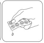
Add 1 Permanganate Value tablet(s). (Into the first test tube.)
