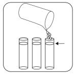
Fill up three test tubes with sample to the 100 mL mark.
