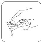
Add 2 Permanganate Value tablet(s). (Into the second test tube.)
