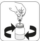
Add Alkalinity Reagent ALK3 or Alkalinity Reagent ALK4 drop by drop to the sample until discolouration turns from pink to colourless.
