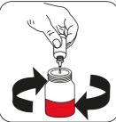
Add Alkalinity Reagent ALK3 or Alkalinity Reagent ALK4 drop by drop to the sample until colouration turns from colourless to red.
