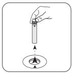
Remove **vial** from the sample chamber.
