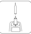
Place the ampoule in the sample chamber.
