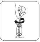
Crush tablet(s) by rotating slightly.
