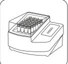
heated thermoreactor for 30 minutes at 100 °C .
