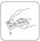
Add **one DPD No. 1 tablet** and **one DPD No. 3 tablet** straight from the foil into the first cleaned cuvette
