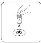
Remove the vial from the sample chamber.
