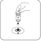
Remove the vial from the sample chamber.
