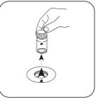
Remove the vial from the sample chamber.
