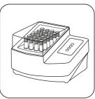
Seal the vials in the preheated thermoreactor for **30 minutes at 100 °C**.
