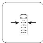
Fill the sample glass to the 25 mL mark with the sample.
