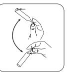
Invert the ampoule several times, allowing the bubble to move from one end to the other. Dry the outside.
