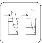
Place a Vacu-vial® ampoule in the sampling vessel. Break off the ampoule tip by applying light pressure against the vessel wall. Wait for the ampoule to fill completely.
