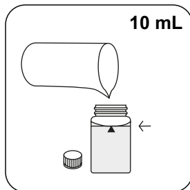
Fill 24 mm vial with 10 mL deionised water .
