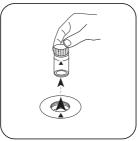
Remove the vial from the sample chamber.
