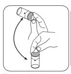
Dissolve tablet(s) by inverting.
