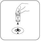
Remove the vial from the sample chamber.
