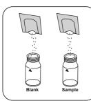
Add a Monochlor FRGT powder pack simultaneously in each vial.
