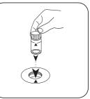
Place Chloramine vial in the sample chamber. • Pay attention to the positioning.
