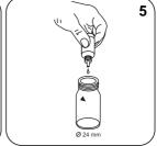
Add 5 drops Free Chlorine Reagent Solution to the Chlorine vial.
