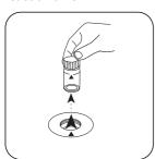
Remove the vial from the sample chamber.
