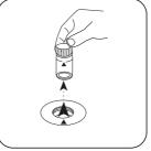
Remove the vial from the sample chamber.
