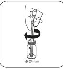
Crush tablet(s) by rotating slightly and dissolve.
