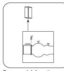
Remove **vial** from the sample chamber.
