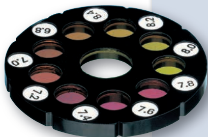
Test disc with colour stable glass standards
