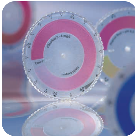
CHECKIT® Discs with continuous and stable scales
