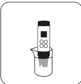
Hold the tester without protective cap in the sample water to be measured so that the electrode and temperature probe is immersed in the sample water not deeper than the seal ring.
