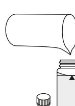
Fill up vial with **sample** to the **10 mL mark**.
